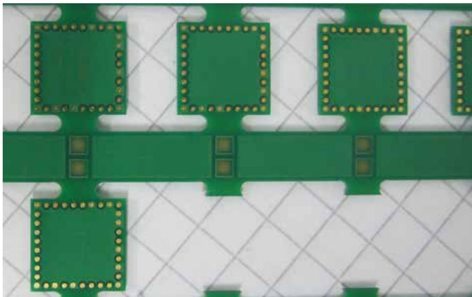
Figure 3: PCB Depaneling with 532 nm laser from InnoLas Photonics
