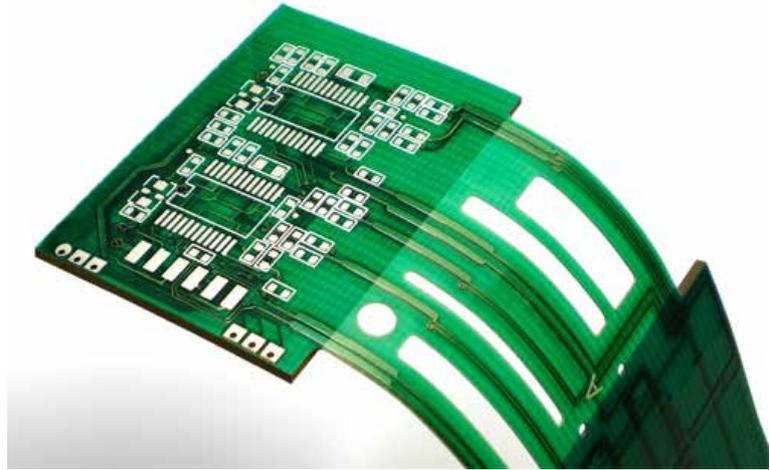
Figure 1: Semi-flexible Rigid-Flex PCB (courtesy Andus Electronic GmbH)
